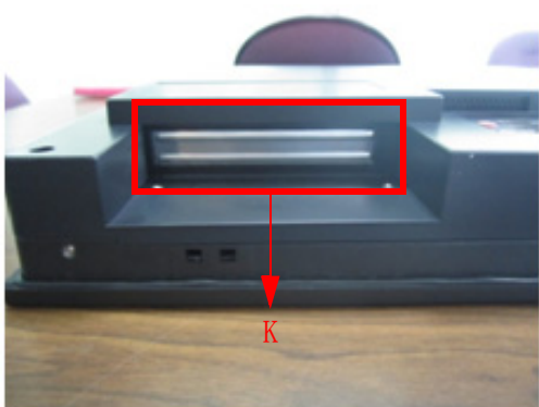
Figure 2.4 PCI expansion slot
