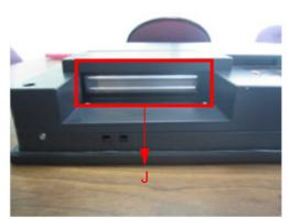
Figure 2.4 PCI/PCIe expansion slot
