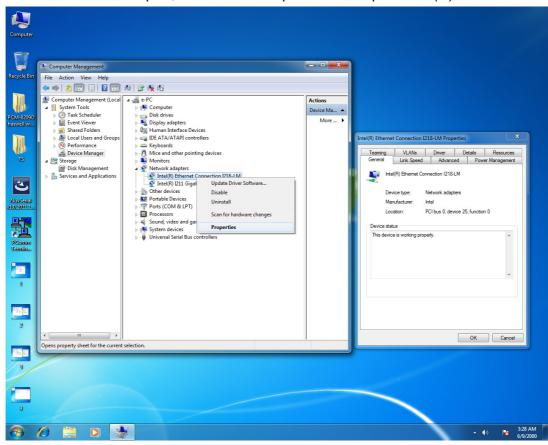
6. Select "Work On Magic Packet", "Work On Pattern Match" and "Work On Magic Packet From Power Off State" under "Power Management".
