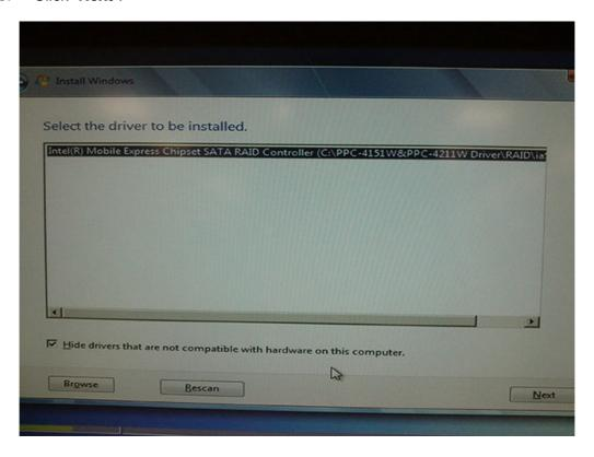
10. Replace the driver disk with system setup disk after installation of RAID driver is finished, then click "**Next**" to return the normal system installation.
