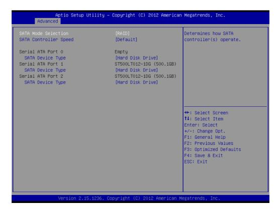
3. Press "Ctrl + I" to enter RAID configuration utility when entering the second start-up screen.
