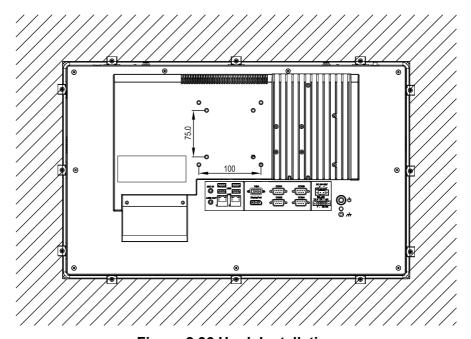
Figure 2.36 Hook Installation
