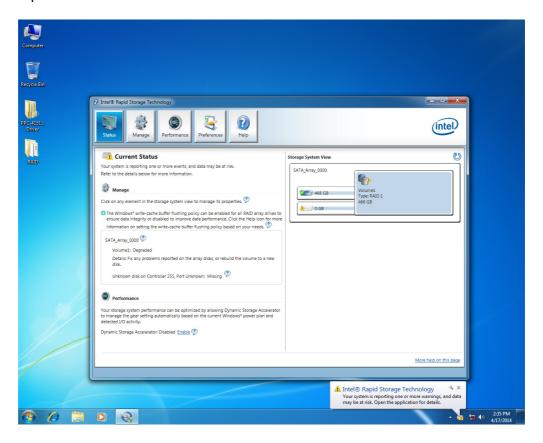
14. At this time, you will need to turn off the computer to change the failed HDD. After entering the system, click "Rebuild to another disk" to back up the system to the new hard disk.
