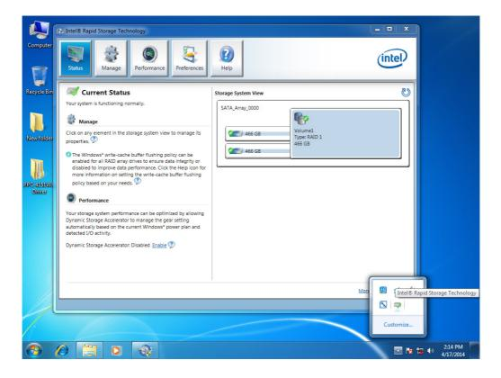
13. If RAID 1 mode is installed and when one the HDDs fails, a pop-up message will appear in the lower right corner. Click the message box to check details of the problem.
