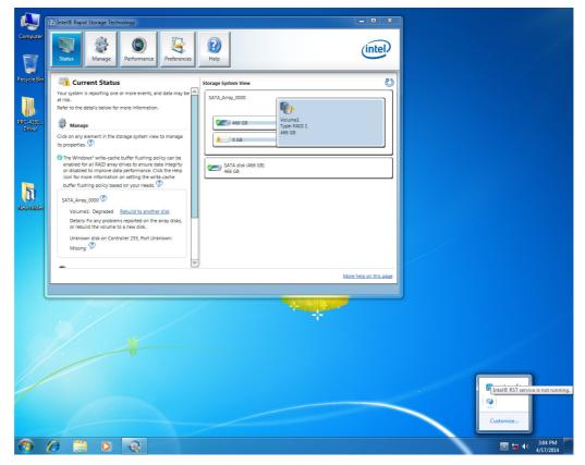
15. When the rebuilding status shows 100%, system backup is complete and RAID 1 function will work again.
