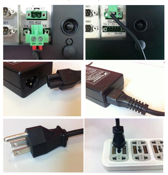
Figure 2.6 Connecting the power cable
