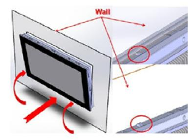
3. Installation is complete as shown in the figure below. Then in the rear of the machine, lock the hook screw and fix the machine according to Section 2.10 "Hook Installation".
