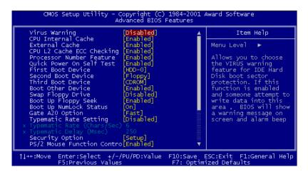
Figure 4.3: Advanced BIOS Features setup
