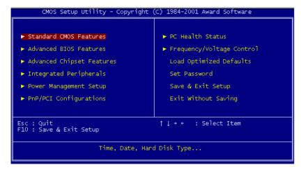
Figure 4.1: BIOS setup program initial screen
