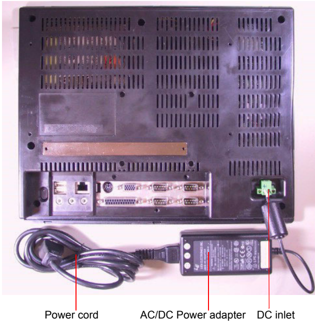
Figure 2.5: Connect the power cord to the DC inlet
