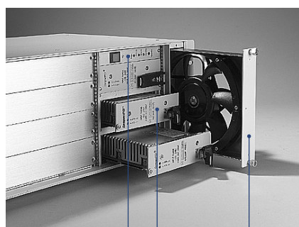
LED board 2+1 redundant CPCI power supply One 193CFM side fan with hot swappable support
