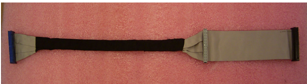
Figure 2.6: Attached IDE 40-pin cable for IPC-7143
