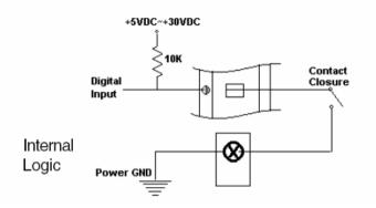
Figure 34: Contact closure input (ADAM-5051/5051D)
