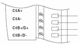
Figure 57: Wiring for Bi-direction Counting
