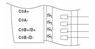
Figure 56: Wiring for Up/Down Counting
