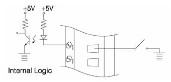
Figure 29: Dry contact signal input (ADAM-5050)
