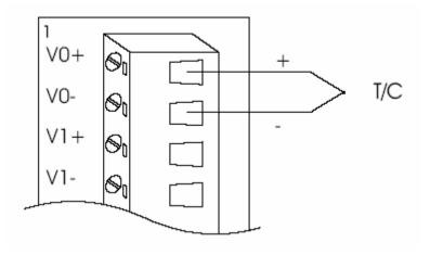
Figure 17: Thermocouple input
