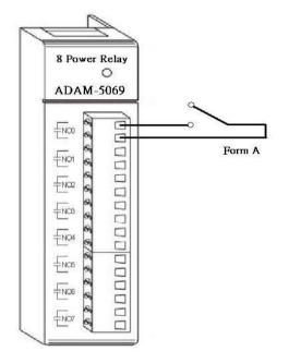
Figure 51: the wiring of ADAM-5069 module frontal view
