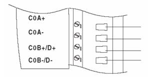
Figure 56: Wiring for Up/Down Counting
