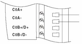
Figure 58: Wiring for Frequency Mode
