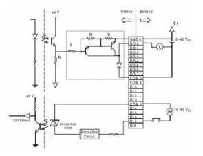
Figure 40: ADAM-5055S module wiring diagram
