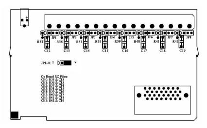
Figure 15: Locations of RC Filter Jumper setting
