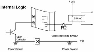
Figure 42: Digital output used with SSR (ADAM-5050/5056)
