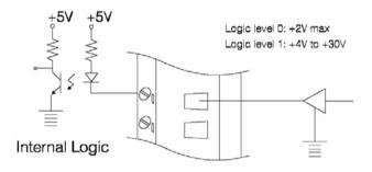
Figure 30: Wet contact signal input (ADAM-5050)
