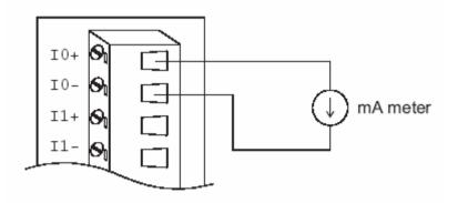
Figure 26: Output module calibration
