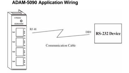
Figure 66: ADAM-5090 Application Wiring
