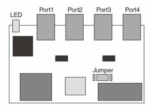
Figure 67: Jumper locations on the CPU card
