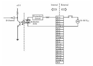
Figure 36: ADAM-5051S module wiring diagram
