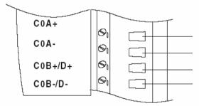
Figure 57: Wiring for Bi-direction Counting
