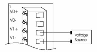
Figure 22: Applying calibration voltage
