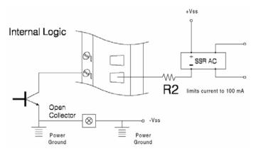
Figure 31: Digital output used with SSR (ADAM-5050/5056)
