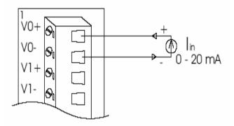
Figure 13: Process current input
