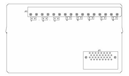
Figure 13: Locations of 125-ohm resistors
