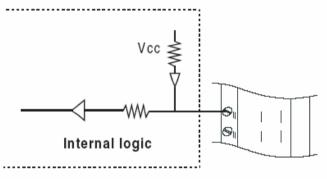
Figure 54: TTL Input Level
