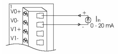
Figure 12: Process current input
