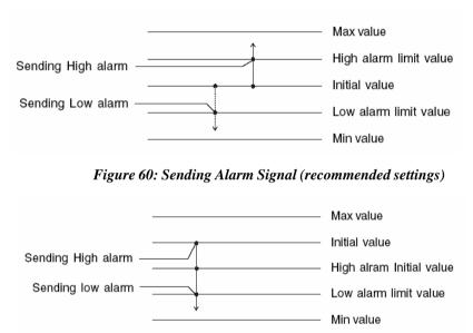
Figure 61: Sending Alarm Signal (settings not recommended)
