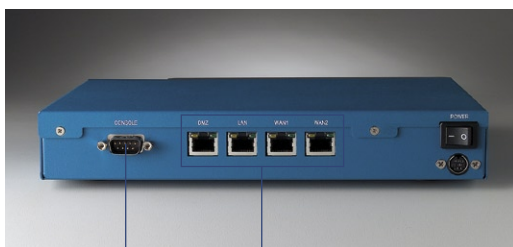
RS-232 console port Four LAN ports
