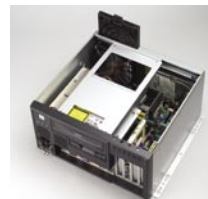
Solid disk drive housing & easy-to-maintain fan filter
