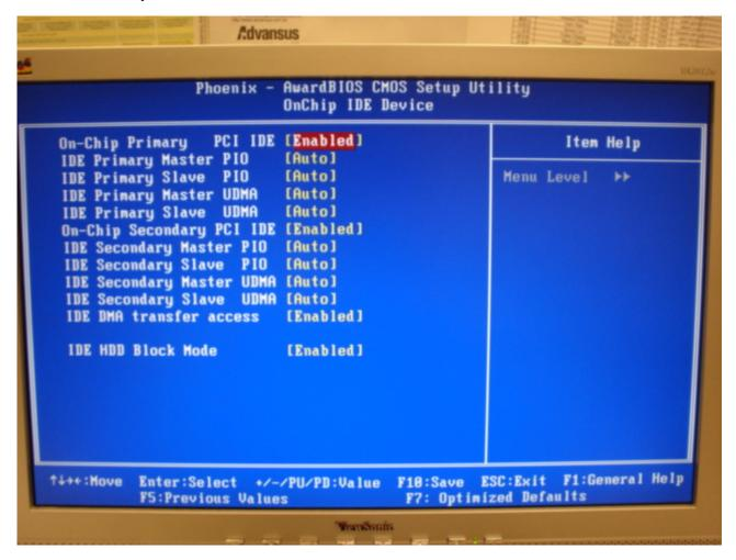
The chipset contains a PCI IDE interface with support for two IDE channels. Select Enabled to activate the primary IDE interface. Select Disabled to deactivate this interface.
