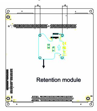
Retention module can be found in the cooler box. Please install the retention module correctly to align with the mark on PCB
