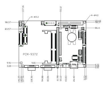
Figure 1.1: Board layout: dimensions
