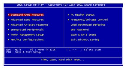
Figure 4.1: BIOS setup program initial screen
