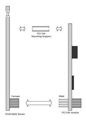
Figure B.1: PC/104 module mounting diagram
