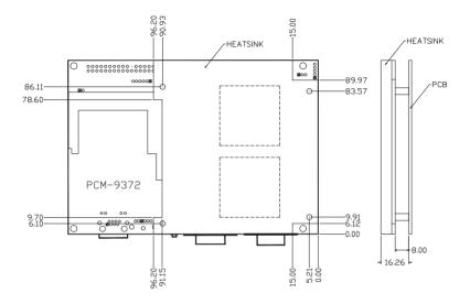
Figure F.2: PCM-9372 Mechanical Drawing (Solder Side)
