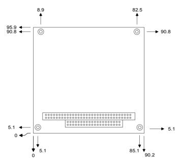
Figure B.2: PC/104 module dimensions (mm) (±0.1)
