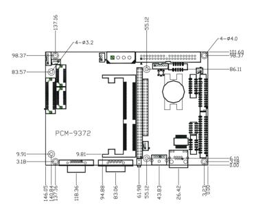
Figure F.1: PCM-9372 Mechanical Drawing (Component Side)
