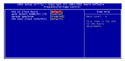
Figure 4.9: Frequency/Voltage Control
