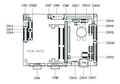
Figure 2.2: Connectors (component side)
