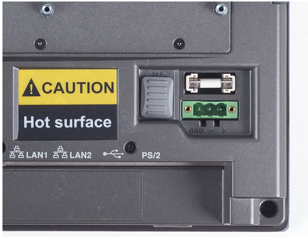
Figure G.1: Fuse Replacement
