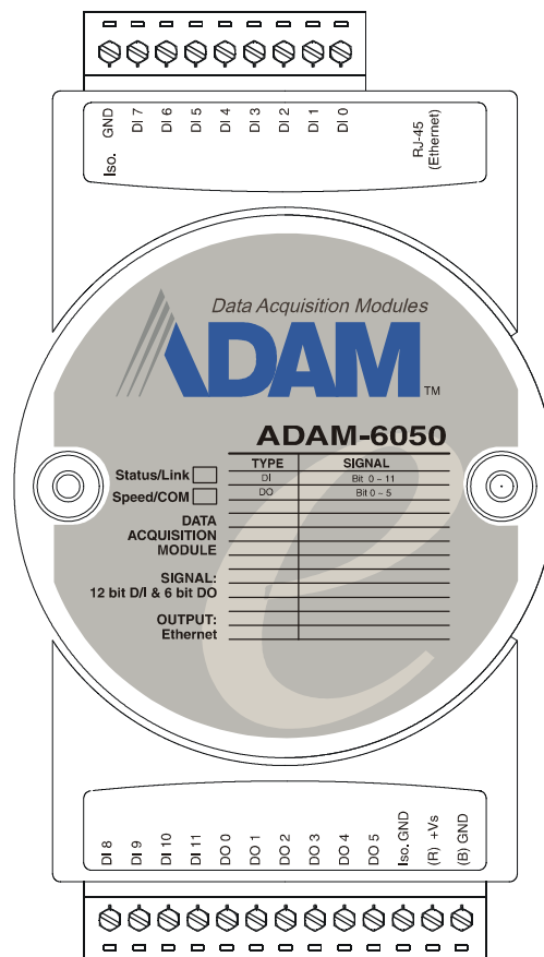
Figure 4-6: ADAM-6050 18-channel Digital I/O Module
