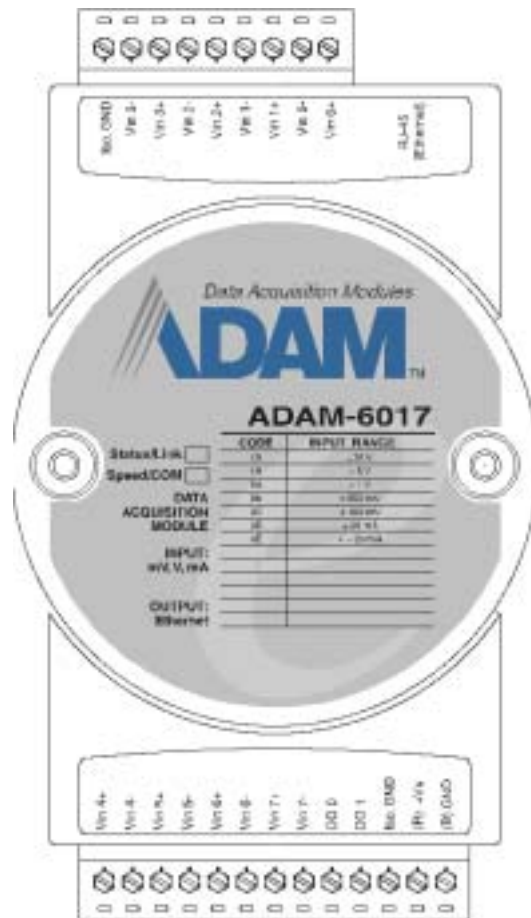
Figure 4-1: ADAM-6017 8-channel Analog Input w/2DO Module
