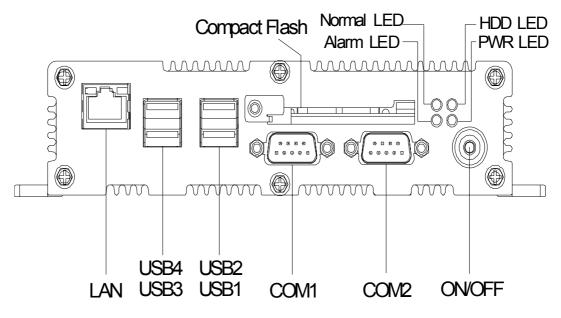
Figure 2.1 ARK-1382 Front Side External I/O Connectors
