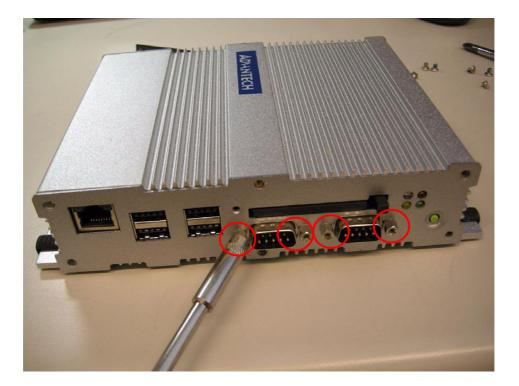
5. Unscrew the 6 screws on the rear panel.
