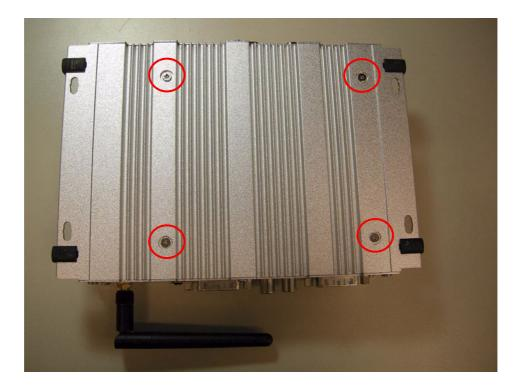
2. Unscrew the 6 screws on the front panel.
