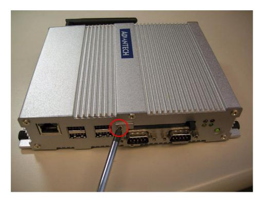
4. Unscrew the 4 hex-bolts on the front panel.
