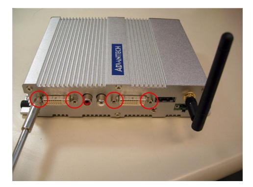
7. Remove the antenna mounting nut.
