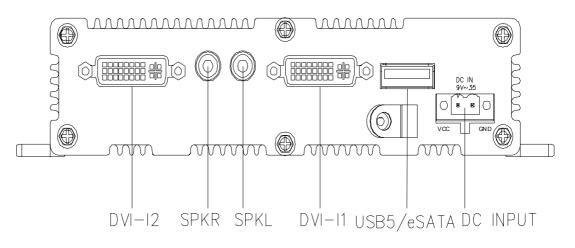
Figure 2.2 ARK-1382 Rear Side External I/O Connectors
