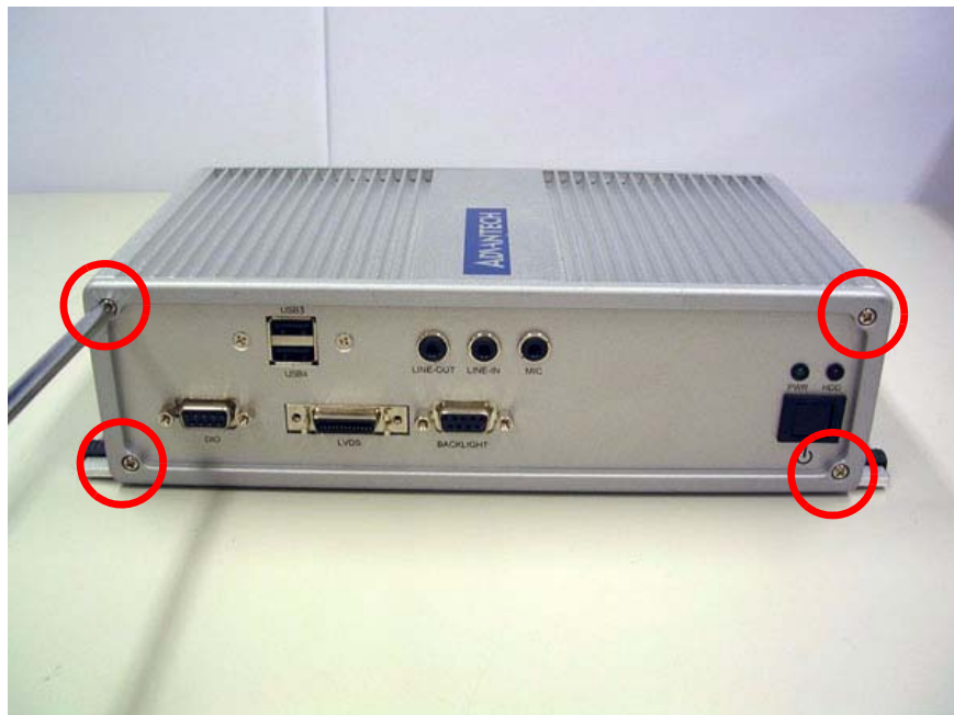
Figure 4.2 Unscrew the frame screws and remove the frame
