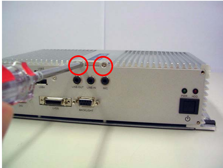
Figure 4.3 Unscrew the panel screws
