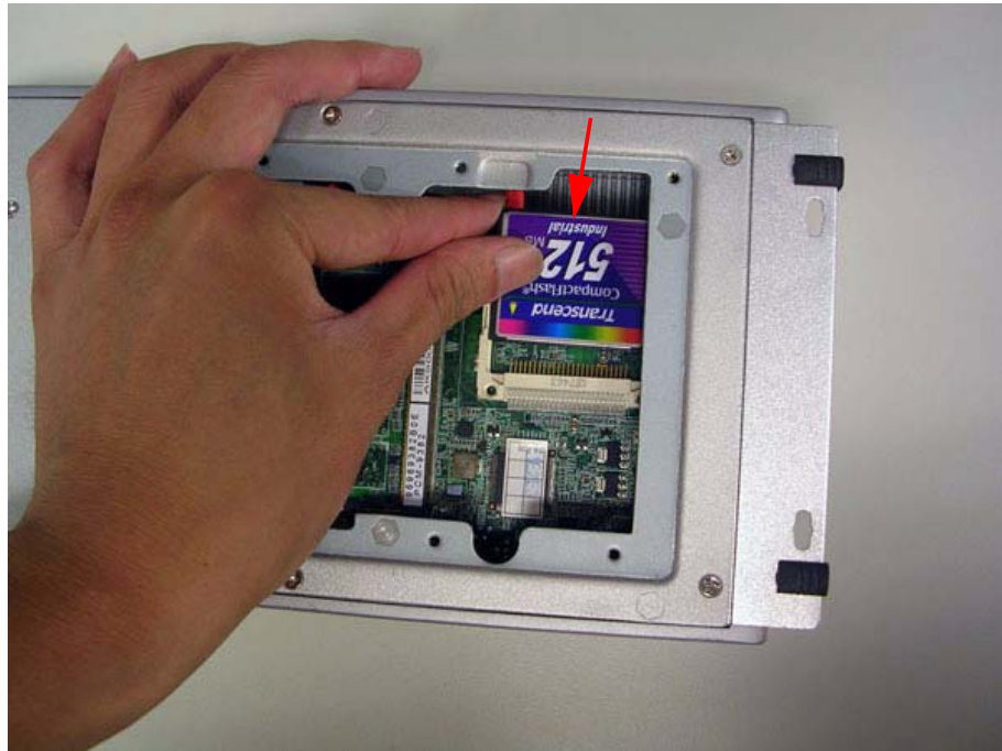
Figure 2.18 Install the CF card into the CF slot at the bottom of the Main board
