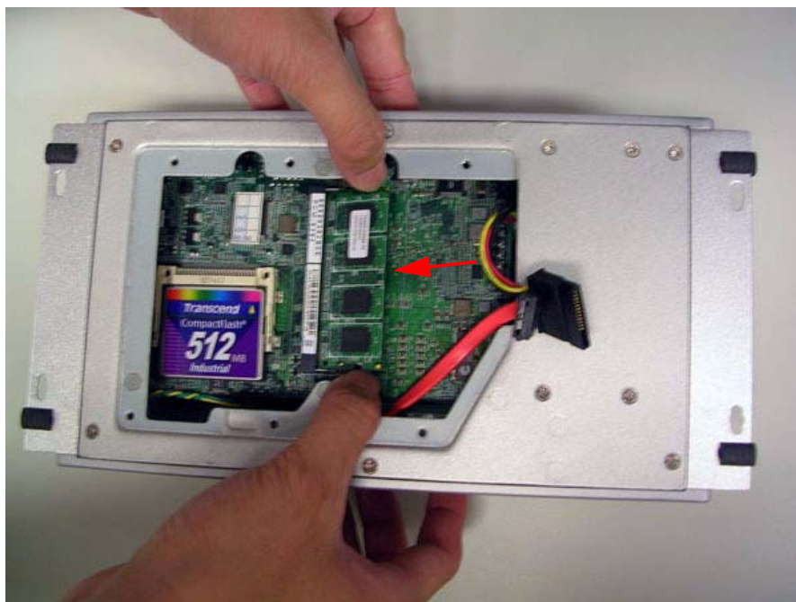
Figure 2.17 Install the memory module into the SO-DIMM socket at the bottom of the Main board
