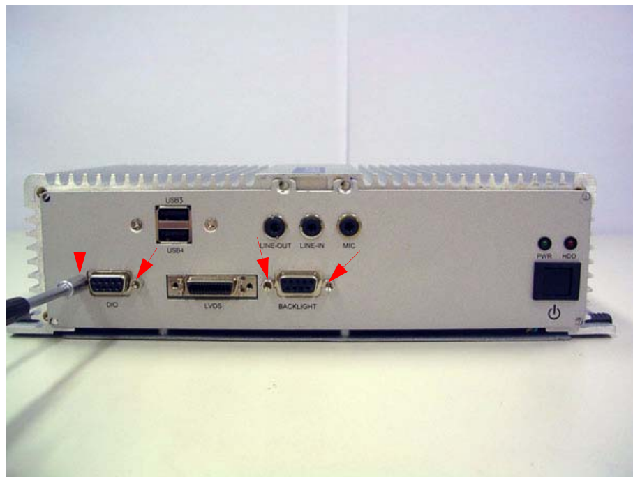
Figure 4.4 Unscrew the hex-bolts on the panel
