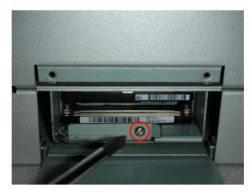
Figure 2.18 Secure the HDD housing with screw
