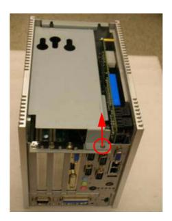
Figure 2.20 Unscrew and remove the top bracket
