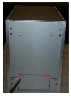
Figure 2.14 Unscrew the HDD door screws
