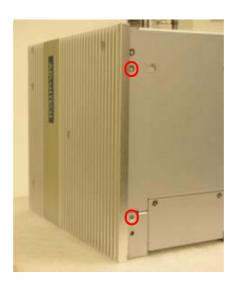
Figure 2.22 Unscrew four screws from back cover
