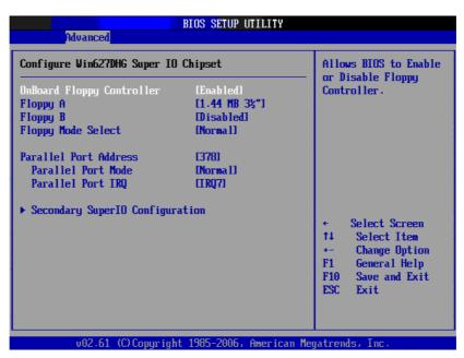
Figure 3.6 Super I/O Configuration
