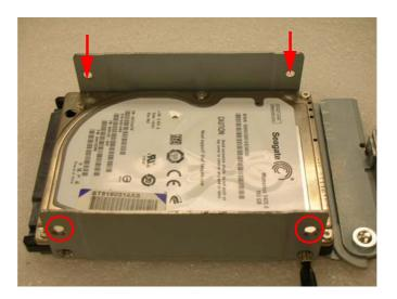
Figure 2.16 Assembly 2.5" SATA HDD and HDD bracket
