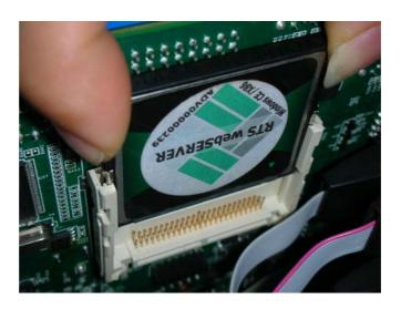
Figure 2.21 Install the CF card
