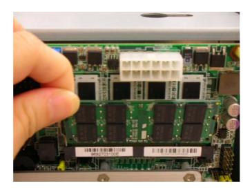
Figure 2.24 Insert the memory module into the SO-DIMM socket
