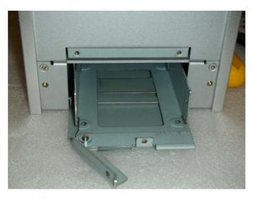
Figure 2.15 Pull out the HDD bracket
