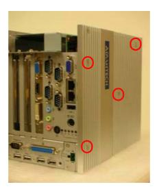
Figure 2.23 Unscrew 4 screws and remove the right side cover
