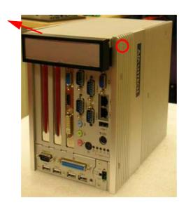
Figure 2.19 Unscrew 2 screws and remove the top cover
