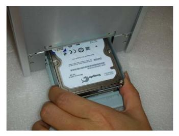
Figure 2.17 Insert the bracket into the HDD housing
