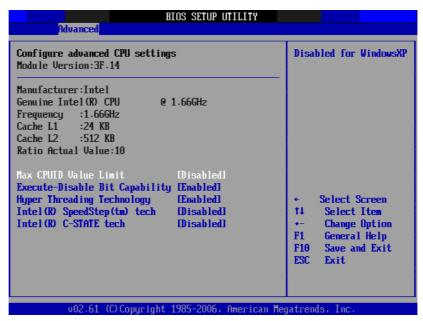
Figure 3.4 CPU Configuration Settings
