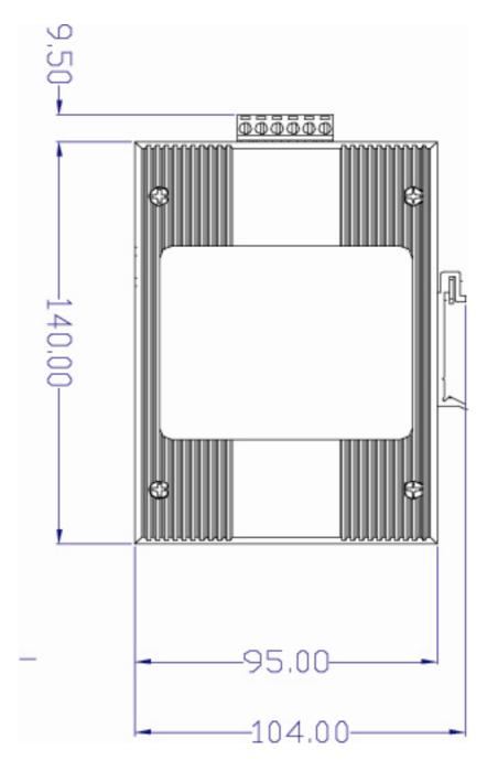
Figure 2.2: Side View of EKI-2701PSI series
