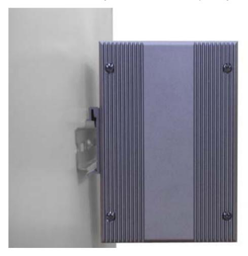
Figure 2.7: Installation to DIN-rail Step 2
