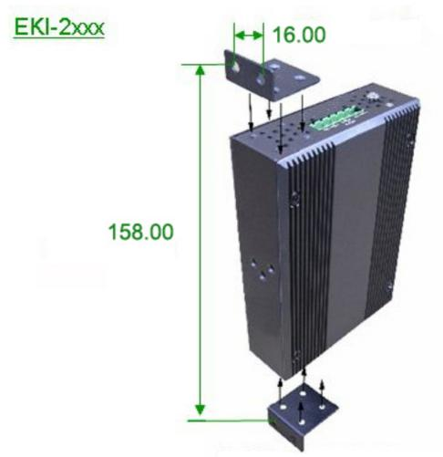
Figure 2.5: Combine the Metal Mounting Kit (units: mm)
