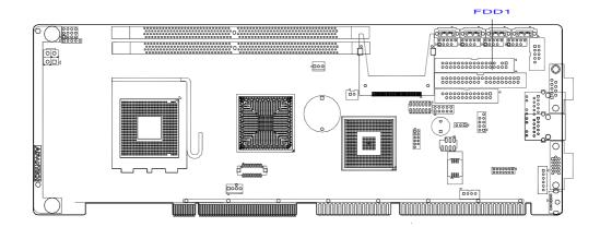
You can attach up to two floppy disk drives to the PCA-6010's on board controller. You can use 3.5" (720 KB, 1.44 MB) drives.
