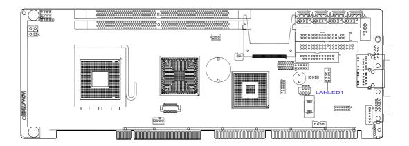
PCA-6010 provides an external LAN LED Pin header for connecting to the front side of the chassis. With this convenient design users can easily see whether the LAN port is active or not. Refer to Appendix B for detailed information on the pin assignments.
