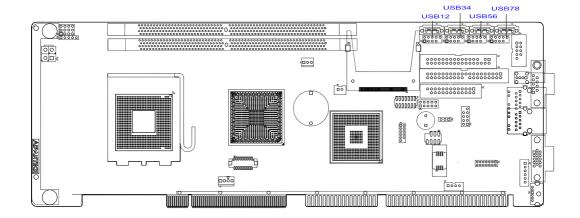
The PCA-6010 provides eight on board USB 2.0 ports which support transmission rates up to 480 Mbps and which are fuse-protected. To install the USB cable (p/n: 1700008461) bracket, find an empty slot in your chassis and unscrew the plate that covers the end of the slot. Screw in the bracket in place of the plate.
