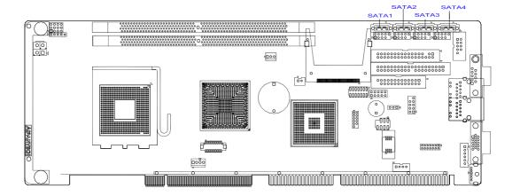
In addition to the EIDE interfaces (up to two devices), the PCA-6010 features a high performance serial ATA2 interface (up to 300MB/s) which eases cabling to hard drives with thin and long cables.
