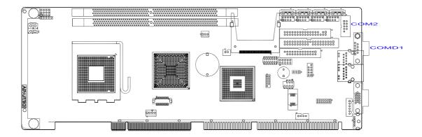
The PCA-6010 offers two serial ports COM1, COM2. These ports can connect to serial devices, such as a mouse or to a communications network.
