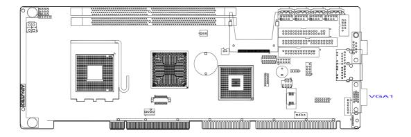
The PCA-6010 includes a VGA interface that can drive conventional CRT displays. VGA1 is a standard 15-pin D-SUB connector commonly used for VGA. Pin assignments for CRT connector VGA1 are detailed in Appendix B.
