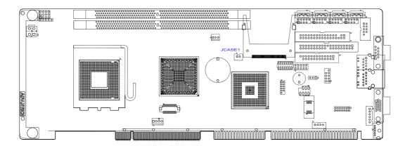
PCA-6010 provides 2-Pins pin header for case open detection. This function could be enabled or disabled in the BIOS setting. When the PIN is shorted, it will cause the on board buzzer to sound.
