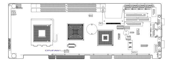
If a fan is used, this connector supports cooling fans of 12 V/1 A (12 W) or less.
