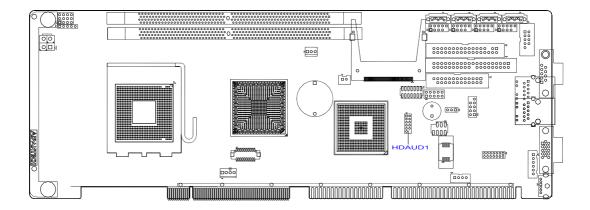
The PCA-6010 provides HD audio through PCA-AUDIO-HDA1 module from Advantech.
