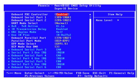
Figure 3.9 Super I/O device
