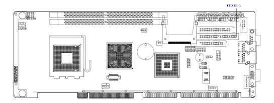
You can attach up to two IDE (Integrated Drive Electronics) drives to the PCA-6010's built-in controller.
