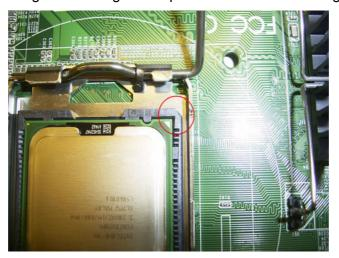
Step 3: Put back the socket cap and press down the bar to fix it.
