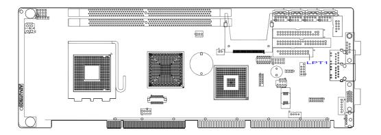
The parallel port is normally used to connect the single board computer to a printer. The PCA-6010 includes an onboard parallel port, accessed through a 26-pin flat-cable connector, LPT1. The card comes with an adapter cable which lets you use a traditional DB-25 connector. The cable has a 26-pin connector on one end and a DB-25 connector on the other, mounted on a retaining bracket. The bracket installs at the end of an empty slot in your chassis, giving you access to the connector.
