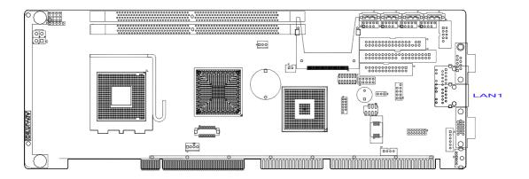
PCA-6010 uses the Intel 82574L Gigabit LAN chip which is linked to PCIe x1 Link. With this chip, PCA-6010 may provide high throughputs for a heavy load networking environment. It provides one or two RJ-45 connectors in the rear side and is convenient for most industrial applications.
