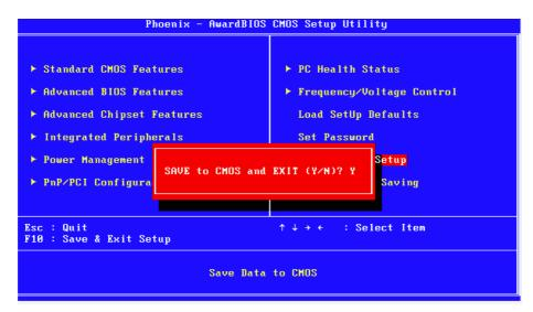
Figure 3.18 Save to CMOS and Exit
