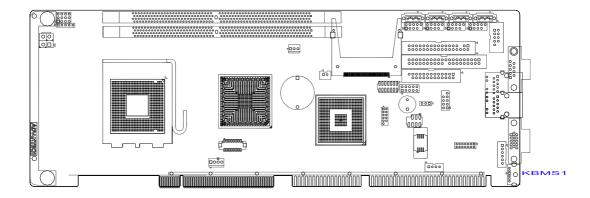
One 6-pin mini-DIN connectors (KBMS1) on the card mounting bracket provide connection to a PS/2 keyboard or a PS/2 mouse, respectively. KBMS1 can also be connected to an adapter cable (P/N: 1700060202) for connecting to both a PS/2 keyboard and a PS/2 mouse.
