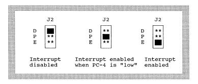
Fig. 2.3 Interrupt Enable selection
