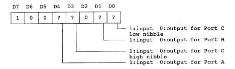
Fig. 3.2 CFG register format (mode 0)
