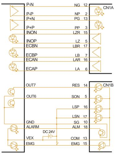
Figure D.1: Wiring Diagram with Mitsubishi MR-J2S Series Motor Driver
