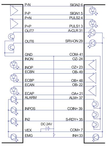
Figure D.3: Wiring Diagram with Panasonic MINAS-A Series Motor Driver
