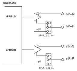
Figure 3.3: Output Signal Loop for Drive Pulses
