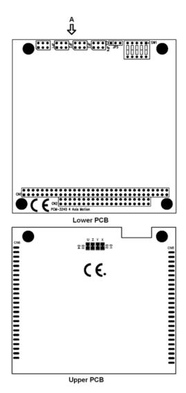
Figure 3.2: Location of Jumpers and DIP switch on PCM-3240
