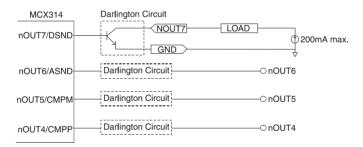
Figure 3.6: Circuit Diagram for General Purposed Output
