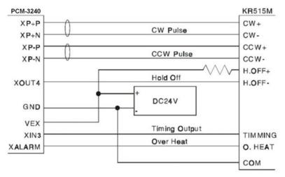
Figure 3.19: Example of Connecting to UPK Step Drive
