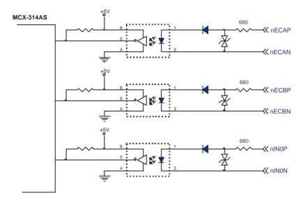
Figure 3.11: Circuit Diagram of Encoder Feedback
