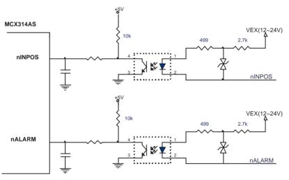
Figure 3.10: Input Signal for Servo Motor
