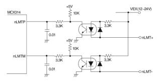
Figure 3.7: Circuit Diagram for Movement Limit Input Signals
