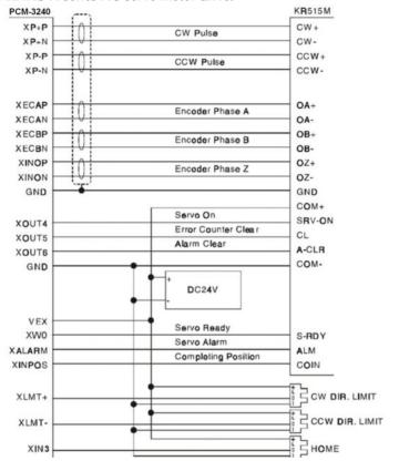
Figure 3.20: Connection Example to MINAS X series AC servo motor drive
