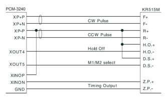
Figure 3.18: Example of connecting to KR515M drive
