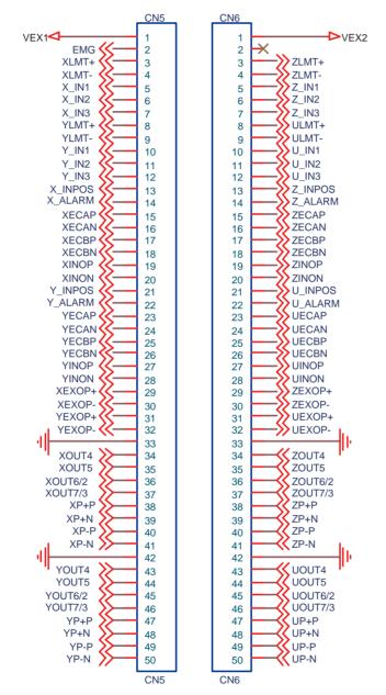
Figure 3.1: I/O Connector Pin Assignments for the PCM-3240
