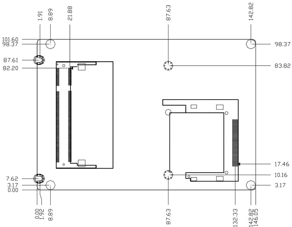
Figure 2.4 Board Dimensions (Solder Side)
