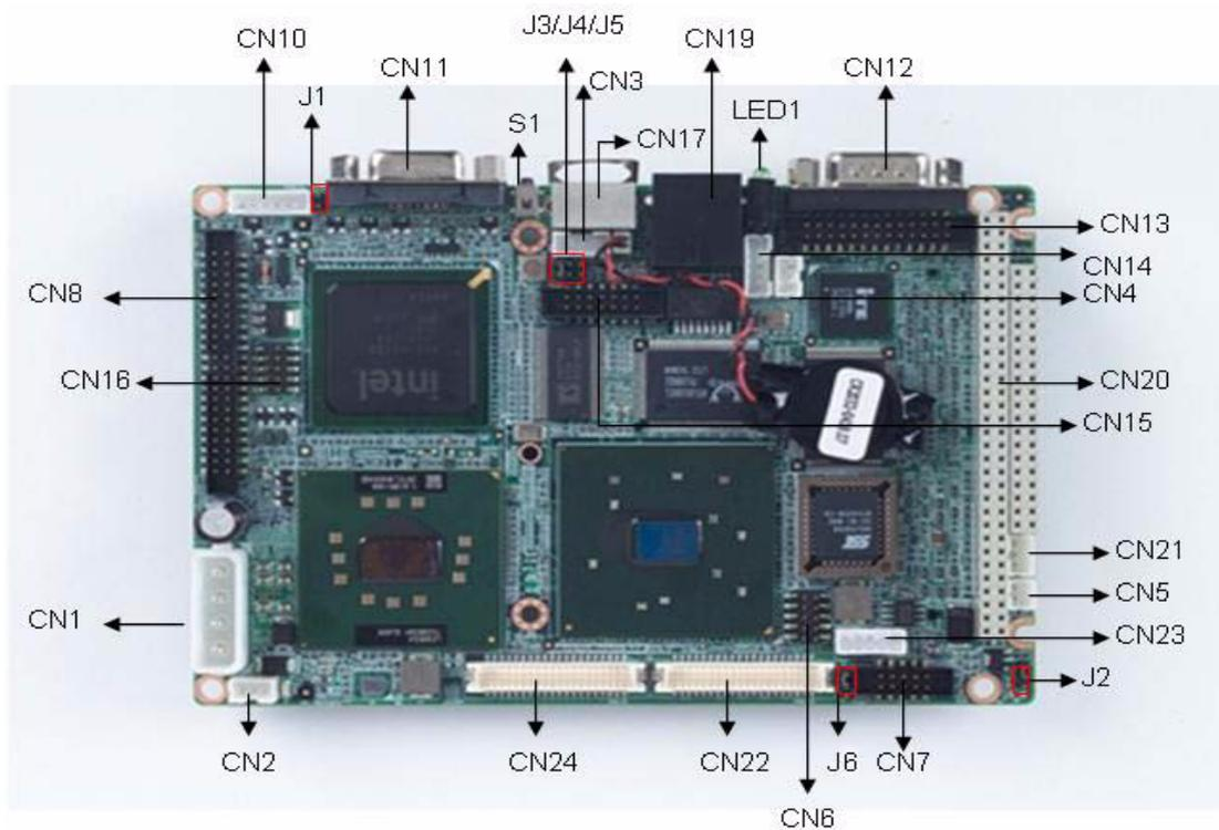
Figure 2.1 PCM-9388 Jumper and Connector Layout (Component Side)
