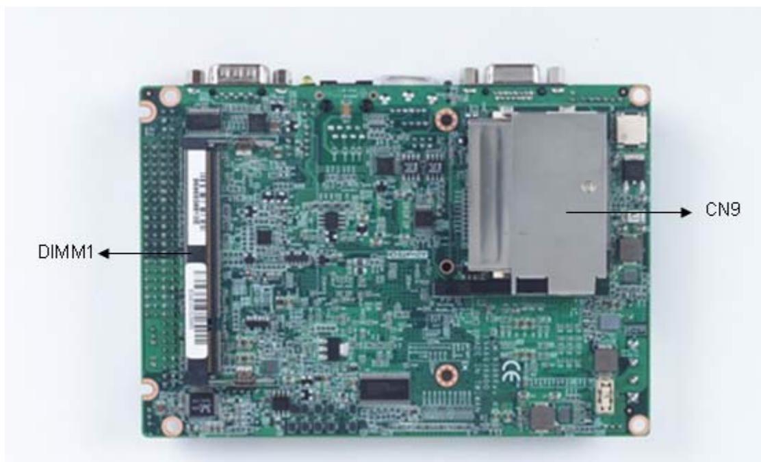
Figure 2.2 PCM-9388 Jumper and Connector Layout (Solder Side)
