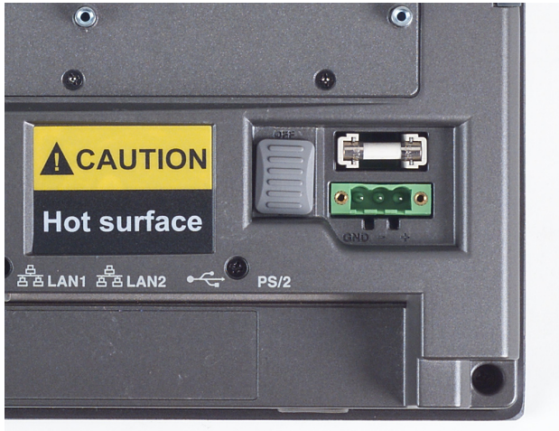
Figure G1: Fuse Replacement
