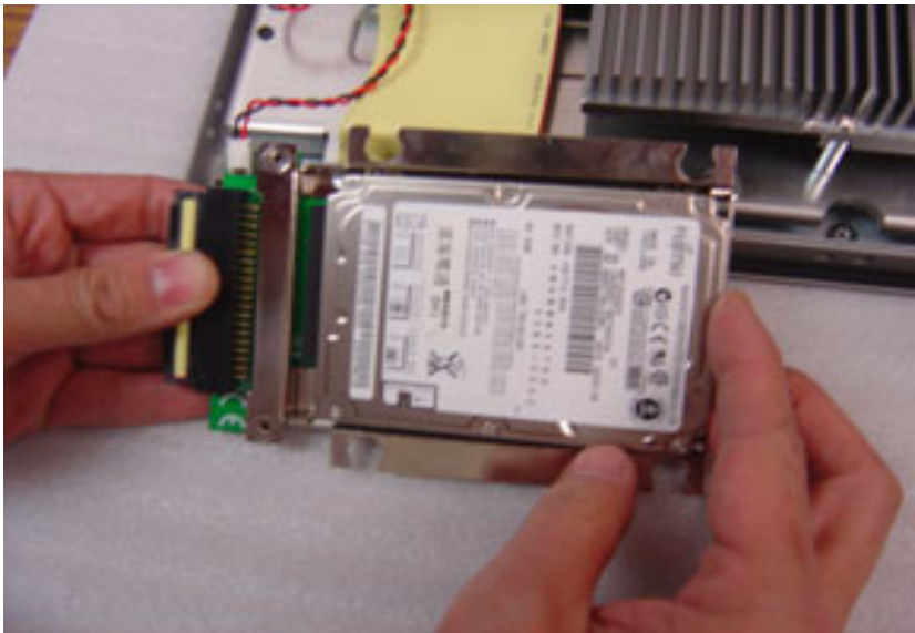
Figure E.6: Installing the HDDr
