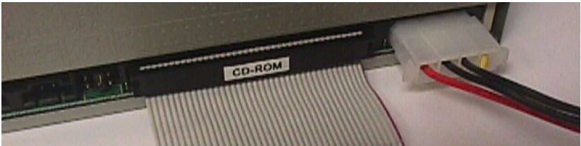
Figure D.7: Plugging in the CD-ROM Drive
