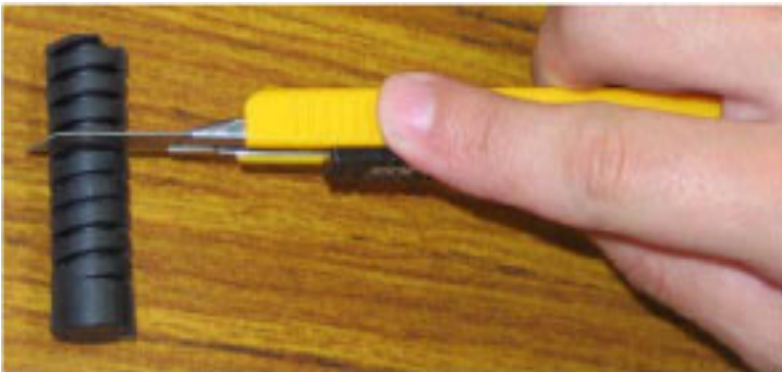
Figure 3.3: Adjust the Anti-Vibration Rubber
