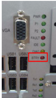
Figure 2.14: LED Location for Battery Backup
