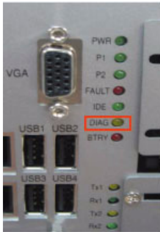
Figure 2.13: LED Location for System Diagnosis
