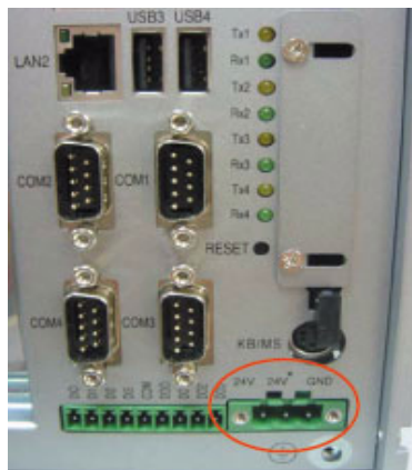
Figure 2.11: Location of Power P1 and P2
