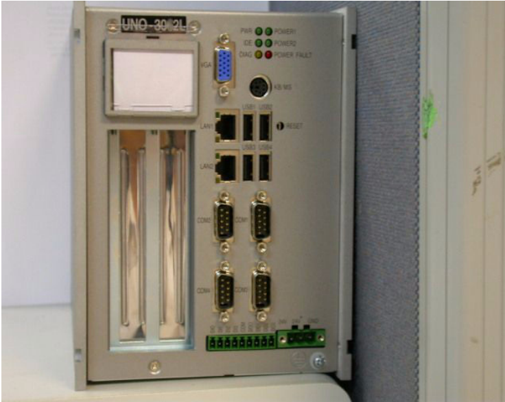
Figure 3.6: UNO-3072L Improper Installation (2)
