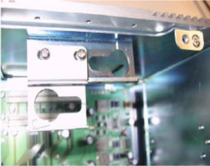
Figure 3.2: 2nd PCI-bus Card Installation
