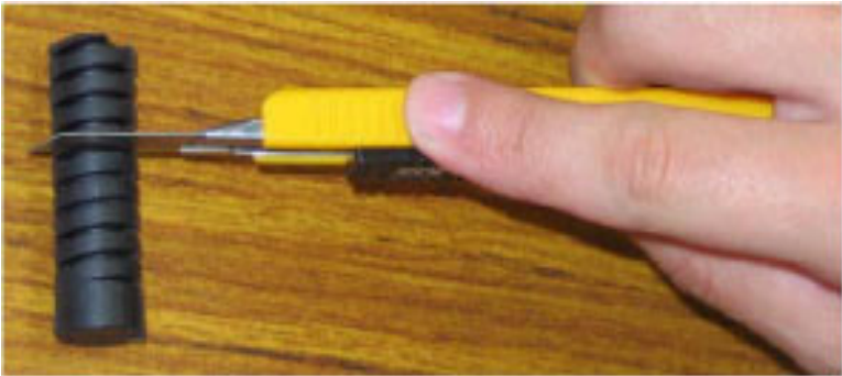
Figure 3.3: Adjust the Size of the Anti-Vibration Rubber
