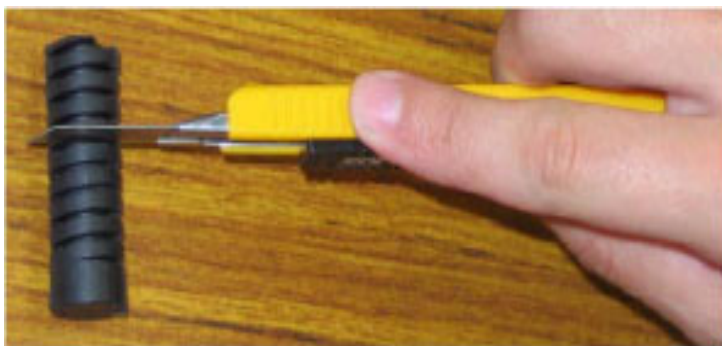
Figure 3.3: Adjust the Anti-Vibration Rubber
