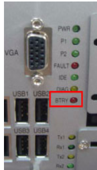
Figure 2.14: LED Location for Battery Backup
