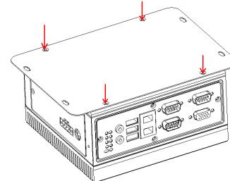
5. Attach the integration kit on FPM using screws according to the table below (p/n: 19330306A0)
