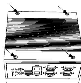
4. Combine the UNO with the VESA mount convert bracket and attach with screws (p/n: 1930001643)
