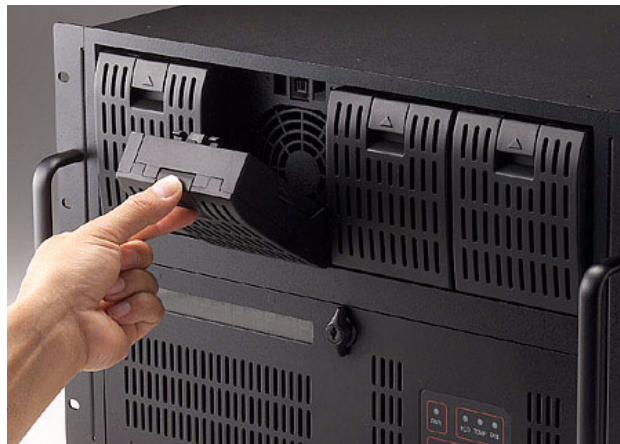
Figure 3.3 Replacing the cooling fan/ 更换热插拔系统风扇 / 更換熱插拔系統風扇
