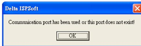
If the communication between ISPSOft and DVP28SV2 fails, please check whether the communication cable comes off, and the setting is incorrect.
