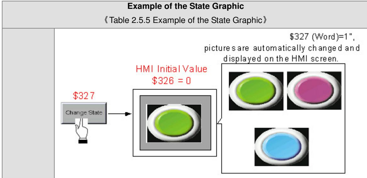
The state graphic supports four data types as shown in the table below. If users need to add or remove state counts, simply add or reduce state counts from State Counts in the properties.
