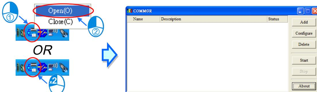
The **COMMGR** window is shown below. The drivers created are listed in the window. ISPSOft connects to COMMGR by means of specifying a driver. Users can manage the drivers through the buttons at the right side of the window. Please refer to the section below for more information about managing drivers.
