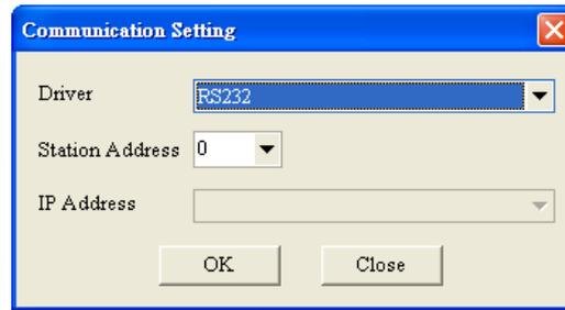
Step 2: After **Upload from PLC** on the toolbar is clicked, the program will be uploaded to the PC.
