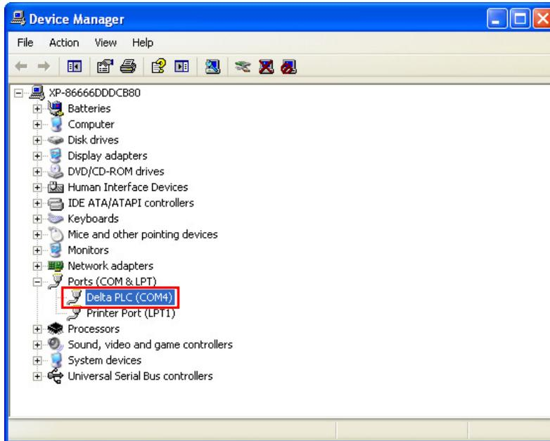
\*. The device name shown in the figure above is the name of an AH500 series CPU module. Different models have different names.
