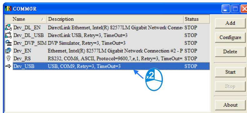
If users want to delete a driver, they have to make sure that the driver stops, select the driver, and click **Delete**, or press DEL on the keyboard to delete the driver.
