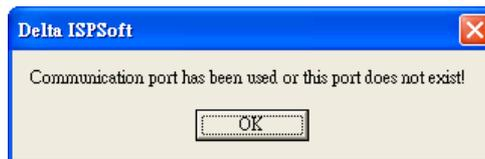
If the communication between ISPSOft and DVP12SE fails, please check whether the communication cable comes off, and the setting is incorrect.
