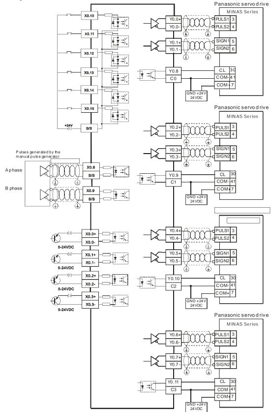
• Wiring AH10PM-5A and a Panasonic MINAS series servo drive
