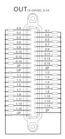
Wiring the external terminal module UB-10-OT32B:
