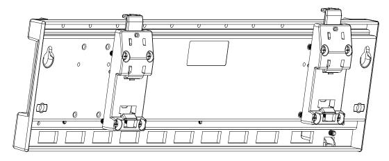
Install the backplane on a DIN rail.
