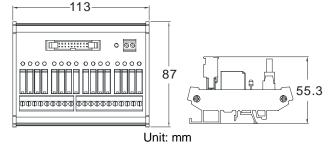
7. External terminal module for AH32AN02P-5C/AH64AN02P-5C: UB-10-OR16B
