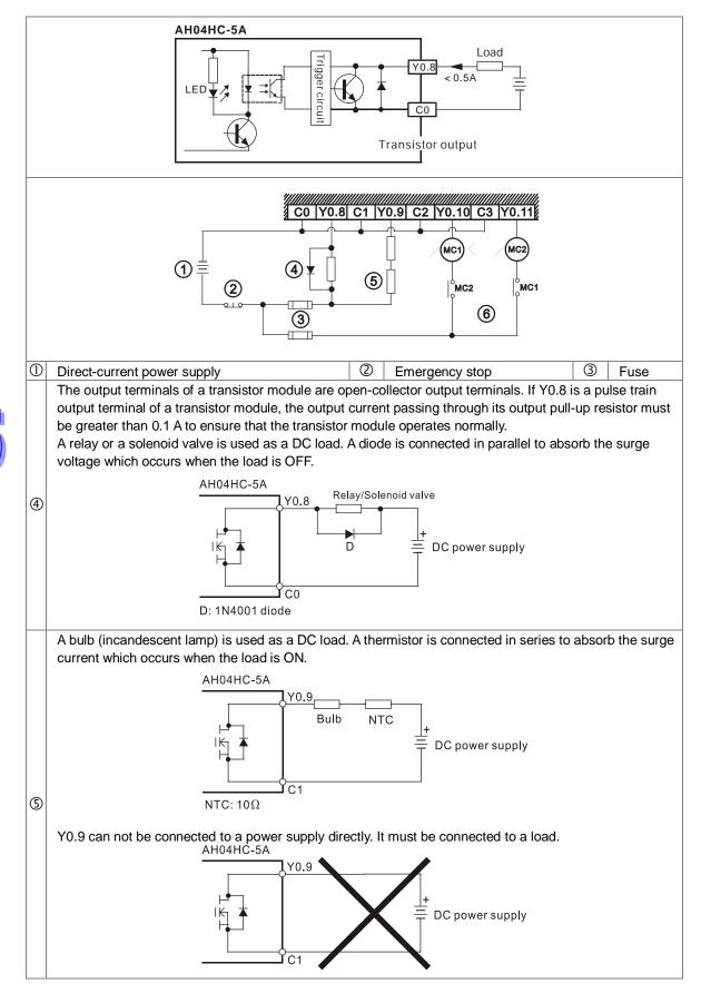
Mutually exclusive output: For example, Y0.10 controls the clockwise rotation of the motor, and Y0.11
