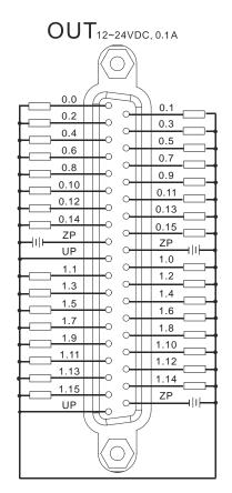
Wiring the external terminal module UB-10-OT32B:
