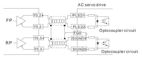
Wiring differential output terminals on AH05PM-5A/AH10PM-5A/AH15PM-5A, and an ASDA-AB series AC servo drive
