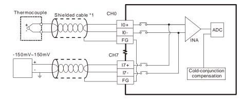
\*1. The cable connected to the input terminal should be the cable or the shielded twisted pair cable which can be connected to type J, type K, type R, type S, type T, type E, or type N thermocouple, and should be kept separate from other power cables and cables which generate noise.
