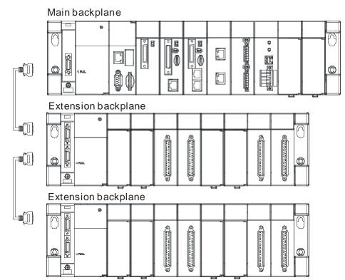
• Fiber optics modules for extension backplanes: AHAADP01EF-5A and AHAADP02EF-5A
