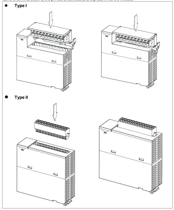
2. Press the clip in the direction indicated by the arrow. Secured the high-dentisy terminal block with screws.
