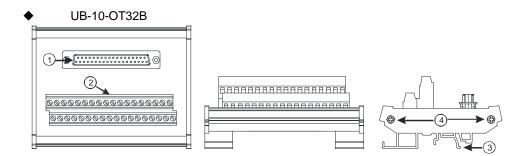
4. External terminal modules for AH32AN02P-5B
