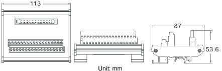
4. External terminal module for AH32AN02P-5C/AH64AN02P-5C: UB-10-OT32A
