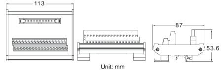
3. External terminal module for AH32AN02T-5C/AH64AN02T-5C: UB-10-OT32A
