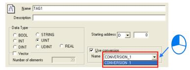
Figure 4-3 Using a conversion
