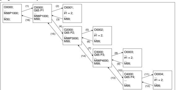
Command G65/G66 can nest macros up to 8 layers. When using with M98 the subprogram call, the maximum layer it can call remains 8.
