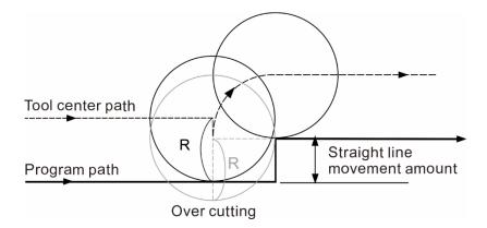
The canceled moving amount of the tool radius compensation must be  $\geq$  the tool radius. Otherwise, there will be interference with the cutting path thus causing excessive cutting. When this issue occurs, the controller will stop running and display the alarm message, as shown in the following figure.
