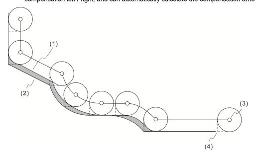
(1) Actual machining contour; (2) Machining contour set in the program;
