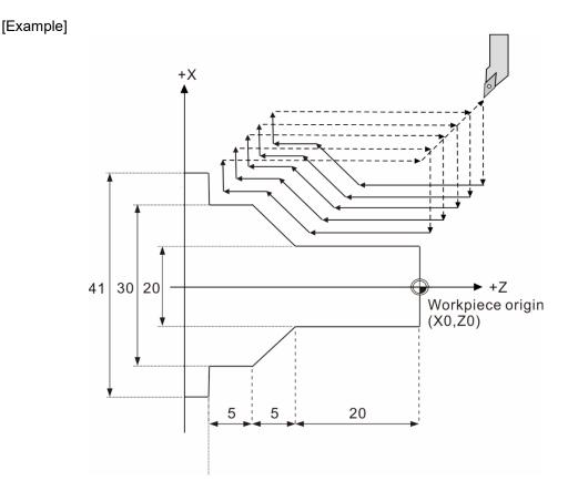
In this program, a bar with diameter 42 mm is used for machining. O0007 M3 S1600 T3 G0 X41. Z2. G73 U10. W10. R5. G73 P50 Q60 U0.4 W0.2 F0.25 N50 G0 X20. G1 Z-20. F0.12 X30. Z-25. W-5. N60 X41. G0 X50. Z10. M5
