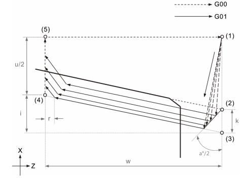
(1) - (5) in the figure represent the tool movement sequence.
