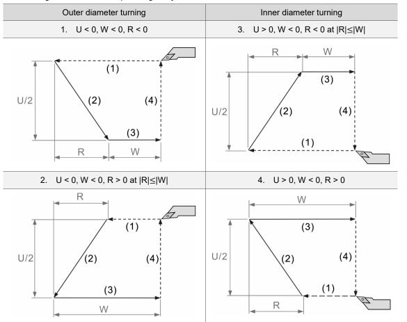
The turning directions corresponding to symbol U, W, and R:
