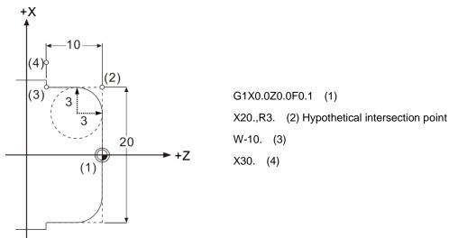
Note: chamfering and corner rounding commands must be followed by a motion block so the chamfering and corner rounding data can be calculated.
