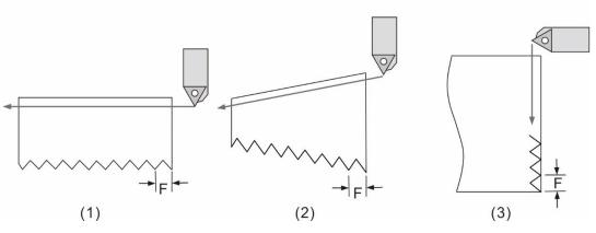
(1) Straight thread; (2) Tapered thread; (3) Scroll thread (face)
