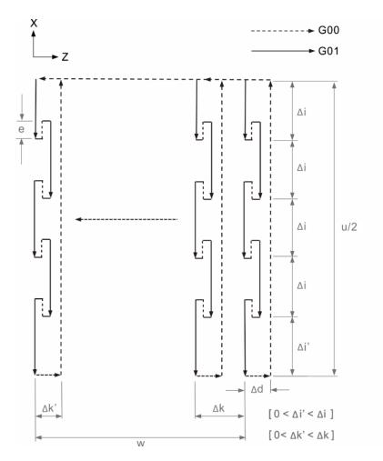
Note: tool nose compensation is not applicable when G75 is used.
