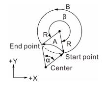
When  $\beta$  > 180°, it means R is a negative value, so arc B is generated. When  $\alpha \leq 180^{\circ}$ , it means R is a positive value, so arc A is generated.
