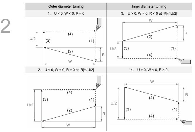
The turning directions corresponding to symbol U, W, and R:
