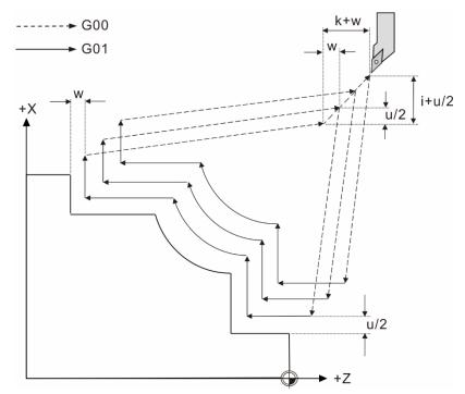
The cutting amount per time: [the total cutting amount of each axis] ÷ [value of cutting times (d-1)]
