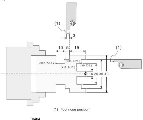
T0404 M3 S2000 G0X30.Z5. (Start point of G74 cycle) G74 R1. G74 X20. Z-5. P3000 Q5000 R0. F0.3 G0X20.Z5. G74 R1. G74 X12. Z-10. P3000 Q5000 R0. F0.3 (Start point of G74 cycle) G0Z5. X50. T0505 G0 Z-18. (Start point of G75 cycle) G75 R1. G75 X30. Z-20. P5000 Q3000 R0. F0.3 G0Z-20. G75 R1. G75 X20.Z-30.P5000 Q3000R0. F0.3 G0 X50. Z5. M5 M30
