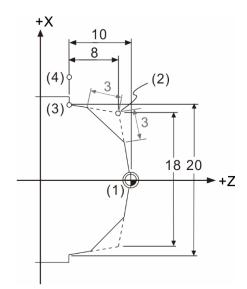
G1X0.0Z0.0F0.1 (1) X18.W-2.,C3. (2) Hypothetical intersection X20.W-8. (3) X30. (4) Format for corner rounding: G01/G02/G03 X/U\_ Z/W\_ ,R\_
