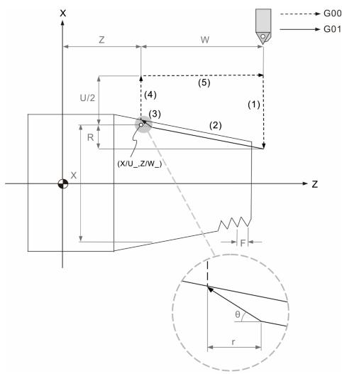
$\theta$  is the chamfering angle for thread turning, which can be specified by machining parameter 349. r is the chamfering length, which can be specified by machining parameter 380. G92 motion analysis:
