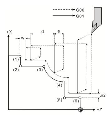
Machining program: G54 X40.0 Z5.0 M03 S1000 G01 X45. Z5. F0.2 G72 W2. R3. G72 P50 Q60 U0.2 W0.0 F0.15 N50 G01 X40. Z-20. (1) X30. (2) Z-15. (3) G03 X20. Z-5. R10. (4) G01 X5. (5) N60 Z0. (6) M5 M30
