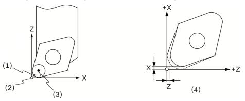
(1) Actual tool nose position; (2) Hypothetical tool nose position when calibration;
