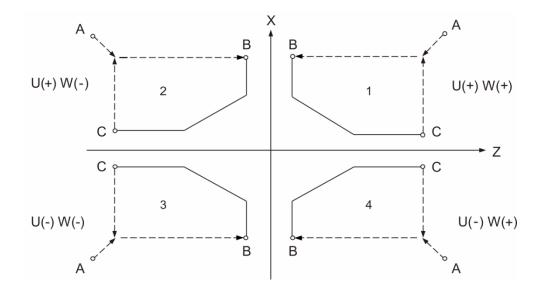
The figure above shows the workpiece position and the cutting direction with respect to the positive / negative U and W values; 1 - 4 represent the four quadrants respectively.
