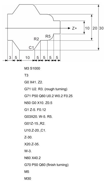
Note: once the G70 finish turning is complete, the tool returns to the start point in rapid traverse and the blocks that follow G70 will be executed.
