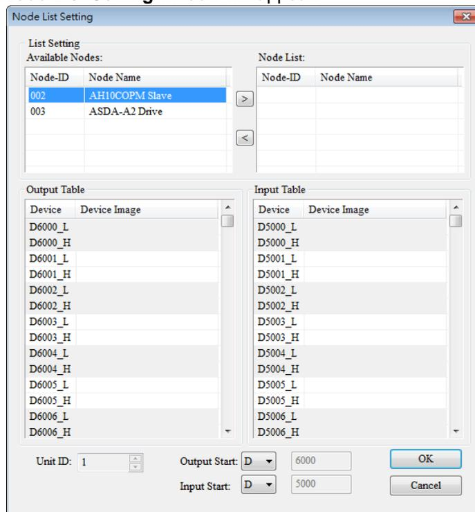
In this example, the ASDA-A2 series AC servo drive whose node ID is 3 is selected. After  is clicked, node ID 3 will be added to the list under **Node List**. When node ID 3 on the list under **Node List** is selected, the data registers in an AH500 series module onto which the I/O data in node ID 3 is mapped are shown in the **Output Table** section and the **Input Table** section.
