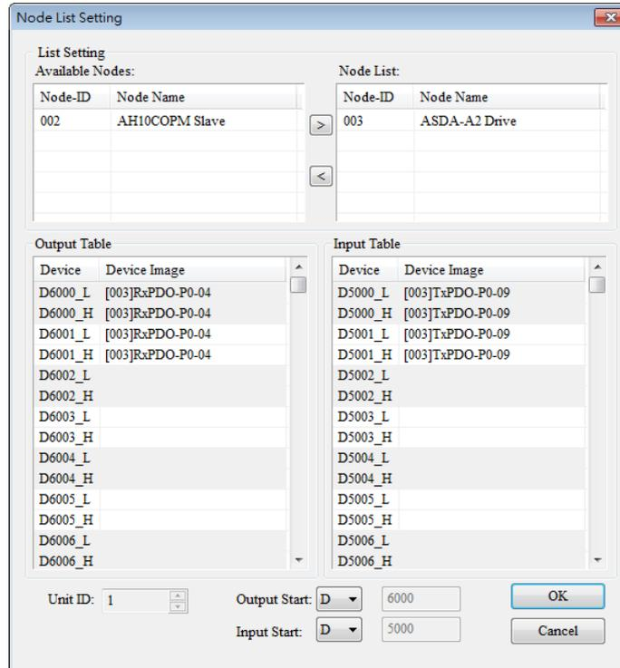
The users can add node ID 2 to the list under **Node List** in the same way. When node ID 2 on the list under **Node List** is selected, the data registers in the AH500 series module onto which the I/O data in node ID 2 is mapped are shown in the **Output Table** section and the **Input Table** section.
