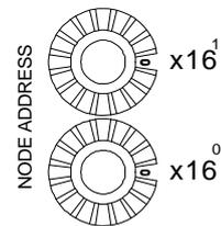
Example: If the station address of AH10COPM-5A is 16#26, users have to rotate the switch corresponding to  $x16^1$  to position 2, and rotate the switch corresponding to  $x16^0$  to position 6.
