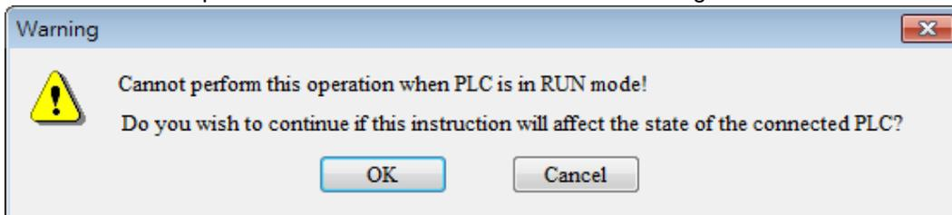
After the users click **OK**, the AH10COPM-5A module will stop running, and the configuration will be downloaded.
