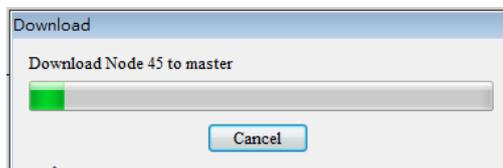
After the downloading of the configuration data is complete, the users will be asked whether they want to run the AH10COPM-5A module again. If the users click **OK** in the **Warning** window, the AH10COPM-5A module will continue operating. If the users click **Cancel** in the **Warning** window, the AH10COPM-5A module will not continue operating.
