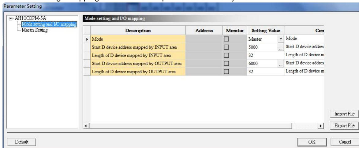
AH10COPM-5A functions as a master station. If the start input address set is D5000, and the start output address set is D6000, the mapping areas assigned will be as described below. The data lengths that the users can set must be in the range of 0 words to 480 words.
