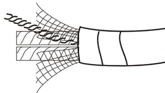
3. After the metallic shield and the foil are removed, the users need to remove the plastic jackets of the power cables and the plastic jackets of the signal cables properly.
