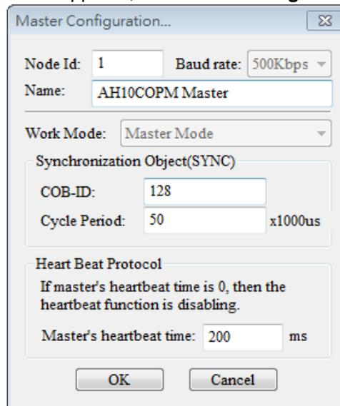
**COB-ID:** Setting the COB-ID used to send synchronous messages
