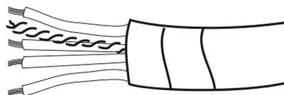
4. Insert the communication cable into the holes in the CANopen connector on AH10COPM-5A, and then tighten the screws on the CANopen connector with a slotted screwdriver.
