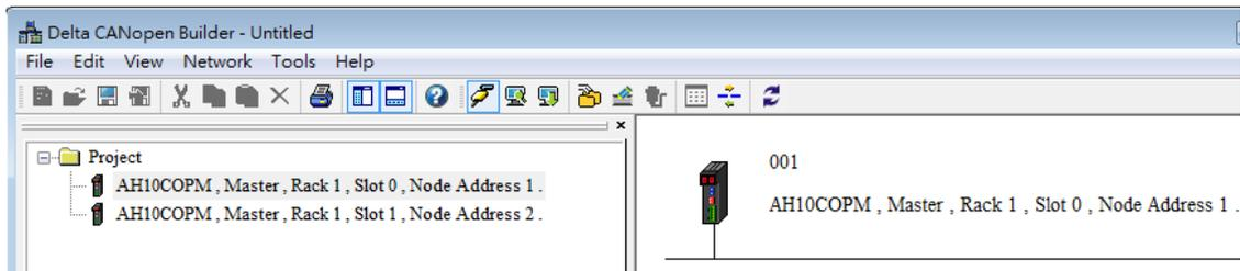
2. After **Online** is clicked, the mode, backplane number, slot number, and node address of the module will be brought out by the software. After the users right-click the master station selected, and click **Scan DeviceNet Network** on the context menu which appears, the information about the node devices on the network created will be scanned.
