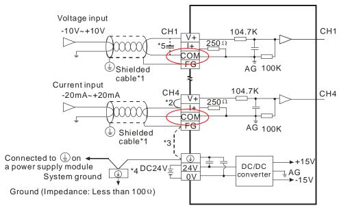
The negative poles of signals are connected to COM, and therefore the cost of wiring terminals is saved.
