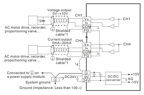
DVP04DA-S2 (DVP04DA-S2 is completely the same as DVP04DA-S. There is no difference in wiring.)
