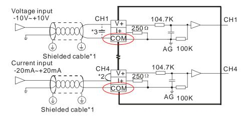
The negative poles of signals are connected to COM, and therefore the cost of wiring terminals is saved.
