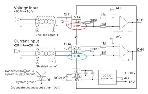
The channels are wired independently, and therefore the noise immunity of DVP06XA-S2 is increased.
