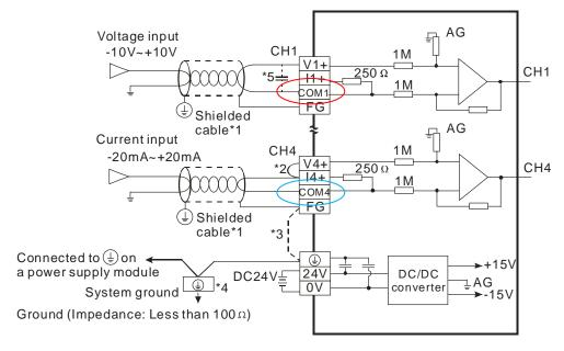
The channels are wired independently, and therefore the noise immunity of DVP04AD-S2 is increased.
