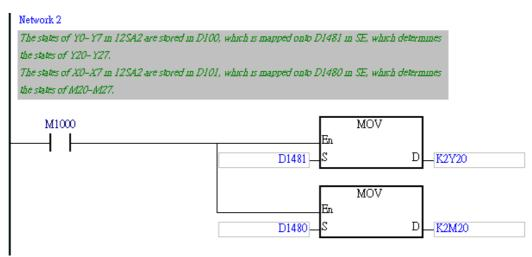
The master station DVP12SE communicates with DVP28SV2 through CANopen. The setting of a high-speed pulse output flag and the setting of a pulse clearing flag are shown below.
