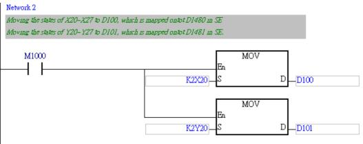
The digital inputs X0~X7 on DVP16SP corresponds to the digital outputs Y0~Y7 on DVP16SP.
