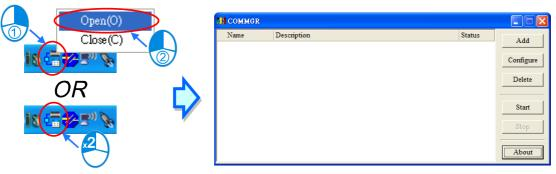
The **COMMGR** window is shown below. The drivers created are listed in the window. ISPSoft connects to COMMGR by means of specifying a driver. Users can manage the drivers through the buttons at the right side of the window. Please refer to the section below for more information about managing drivers.
