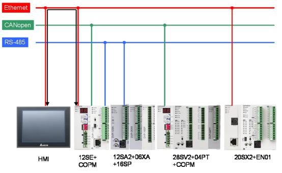
The value in C0 is written into DVP28SV2, DVP12SA2, and DVP20SX2, and then the values written into DVP28SV2, DVP12SA2, and DVP20SX2 are read. The page displayed on the HMI is shown below.
